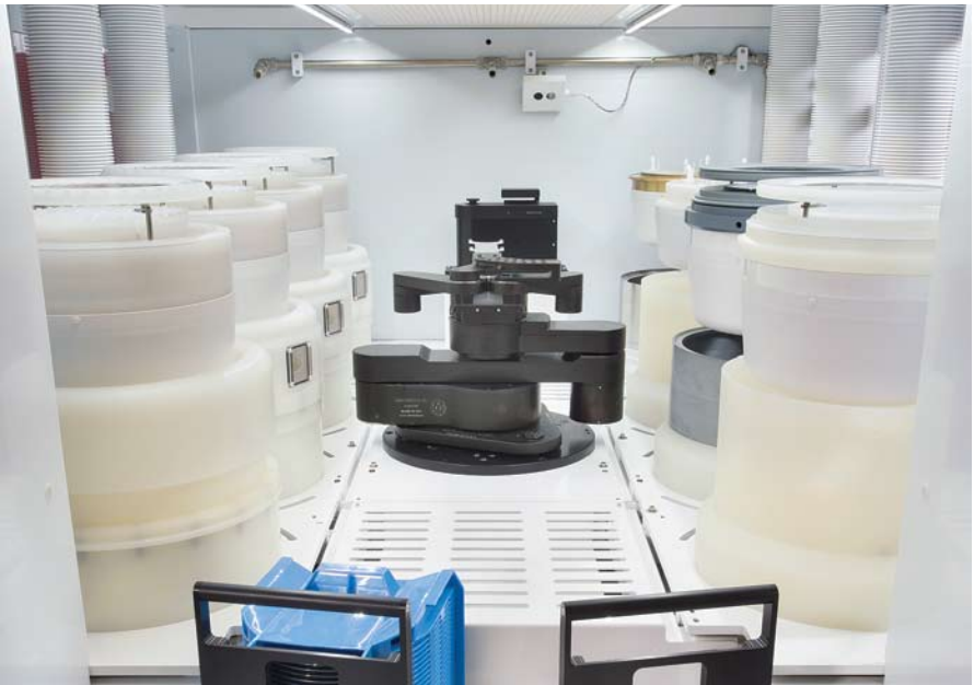
UBM Etch (left) and High Temperature Spray chamber (right) in a Solstice S8 system.
